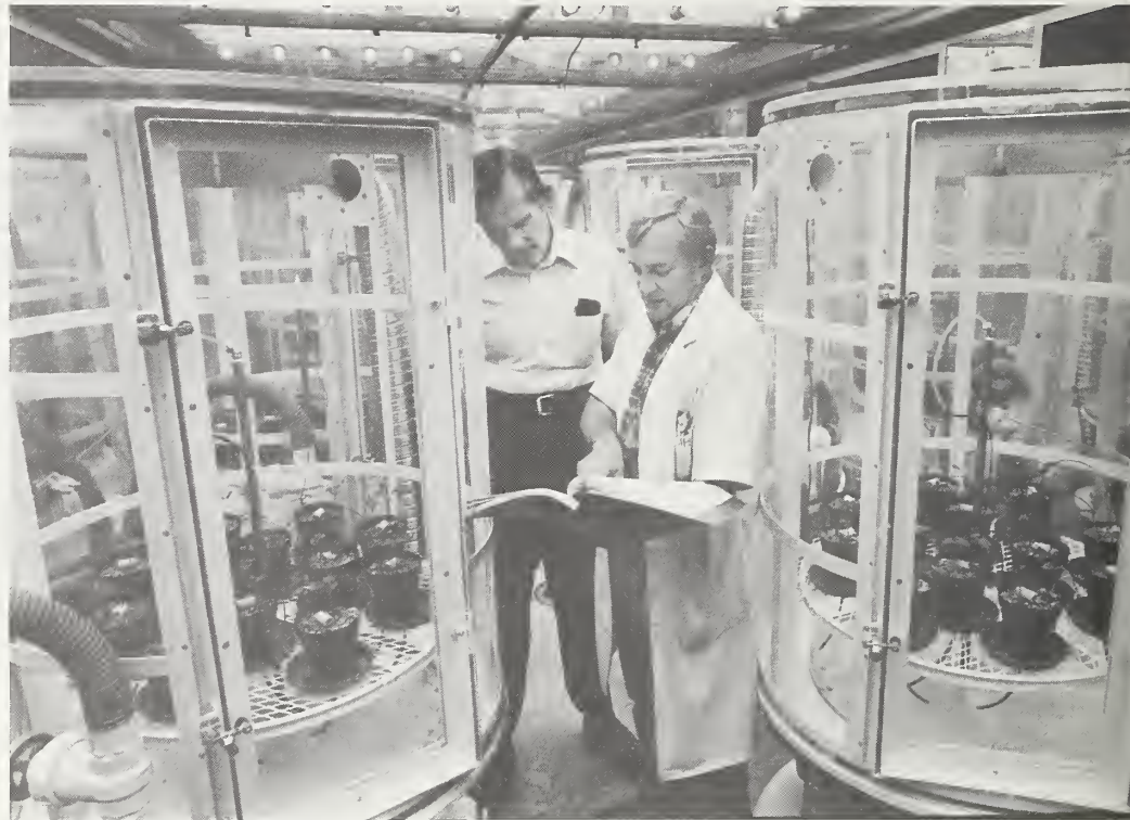
Indoor chambers control environment of snap bean plants to test response to ozone under various conditions. Plant physiologist Walter Heck and botanist John Dunning review records. (0986X1056-6)
